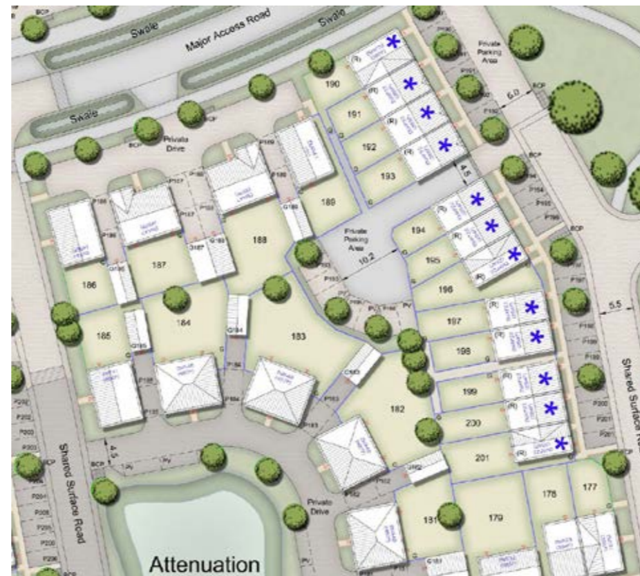
“MIXED” URBAN GRAIN AT THE FRONTAGE OF FORMAL OPEN SPACES AND ALONG THE PRIMARY VEHICULAR ROUTE: LARGER PLOTS / LOOSE URBAN FORM AROUND THE PUBLIC OPEN SPACE SURROUNDING THE LANDSCAPED AREA WITH THE ATTENUATION BASIN, AND A TIGHTER BUILDING FORM AT THE FRONTAGE OF A VILLAGE GREEN.
