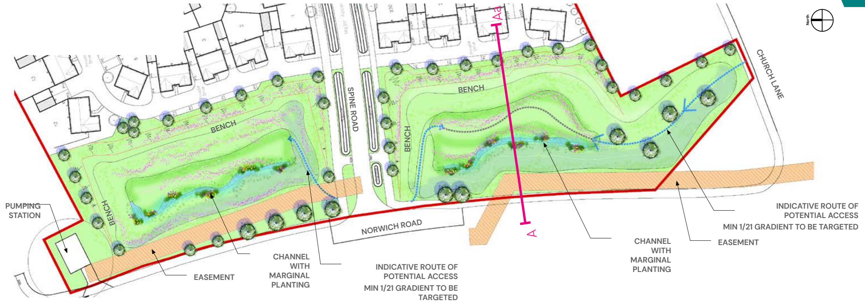
ATTENUATION BASINS ALONG WESTERN SITE BOUNDARY
